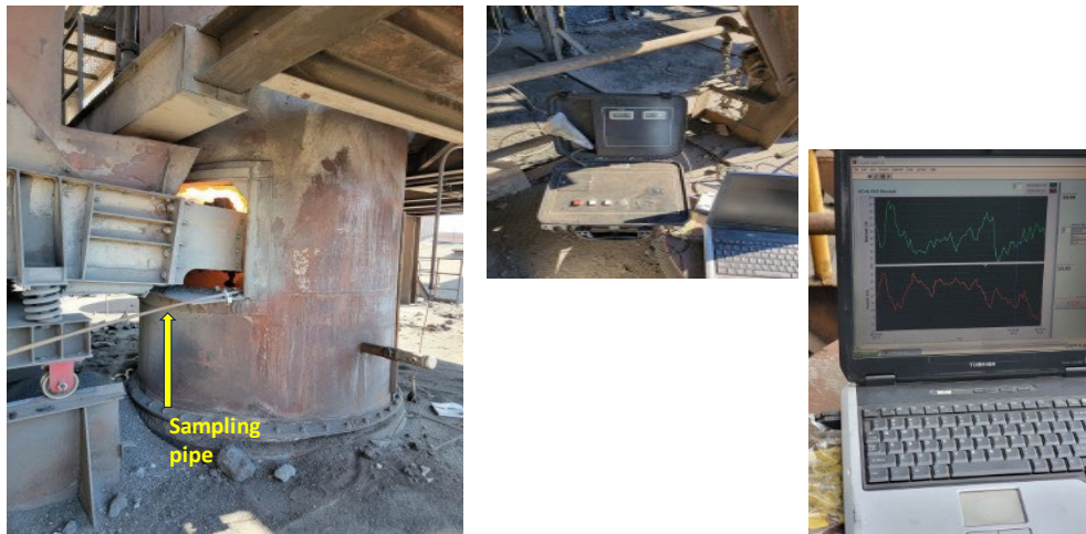
Figure 6. Photos of stack gas sample collection equipment.
